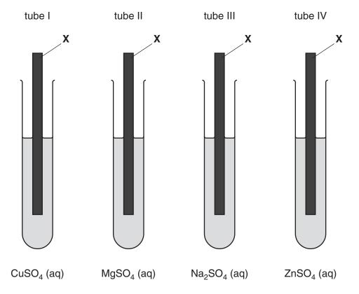
A deposit is formed on metal **X** in only two of the test-tubes.
